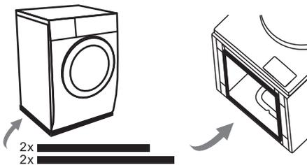
1. Get the machine laid on the floor, using some soft material like foam or clothes between the machine and floor for a protection;
